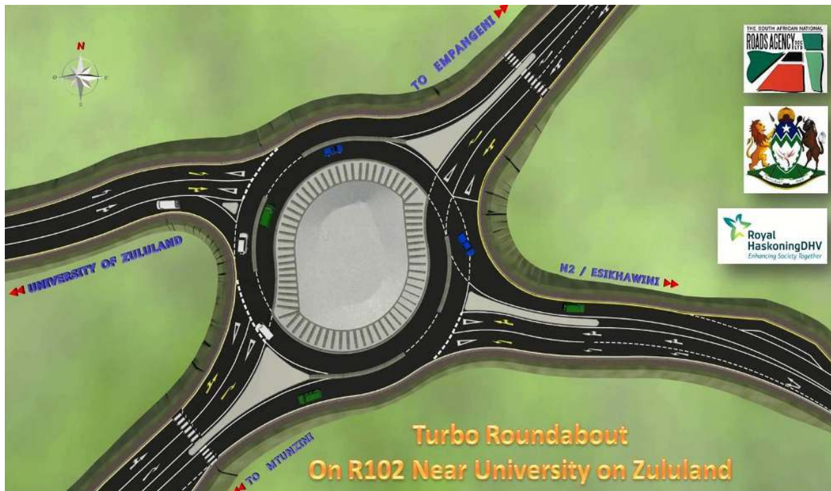
Figure1: Conceptual diagram of the R102 / P535 Turbo Roundabout
