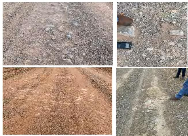
**Figure 5: Material types on the four trial sections. Quartzite (top left), Greywacke (top right), Dorbank (bottom left), Shale (bottom right)**
