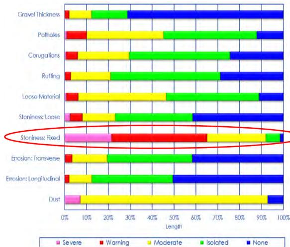
**Figure 1: Defects on the Department's unpaved road network**
