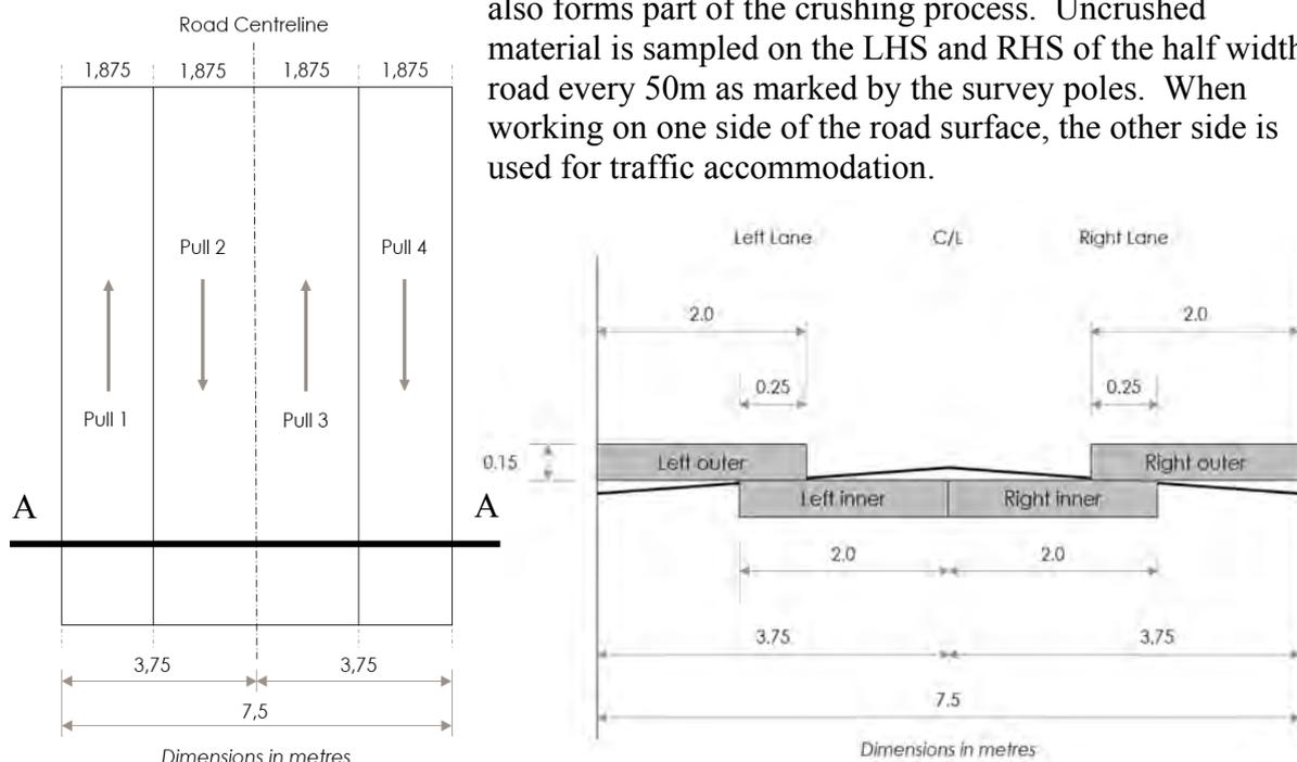
**Figure 6: Layout of crushing process for typical 7.5m wide section(left).
