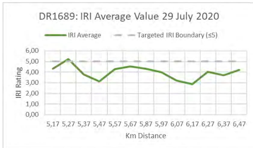
**Figure 11: Average IRI rating for DR1689 test section**
